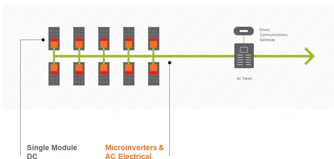
Figure 3: Representation of Enphase Microinverter system
