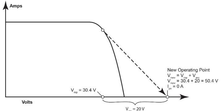
Figure 6: With an arc-fault in series with a working microinverter, the voltage rises to  $V_{mp} + V_{arc}$ . The transfer characteristic of the PV Panel forces the current to zero. With zero current, the microinverter falls off MPPT (Maximum Power Point Tracking) and shuts down.
