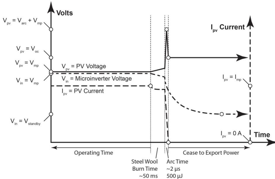
Figure 5: I-V curves explaining the microinverter behaviour during an Arc Fault
